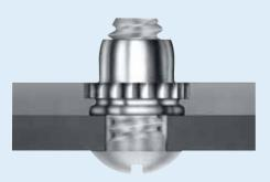
Types FE/FEO/UL elliptically squeezed nuts are self-locking. Types FE/FEO thread locking torque performance is equivalent to applicable NASM25027 specifications. Type UL self-locking nuts meet locking torque requirements specified herein. Some sizes of FE/FEO/UL can be ordered to NASM45938/7 specifications.\*
